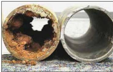
Over the years, iron-oxide (rust) often forms on the inside of unlined pipes. As part of the rehabilitation process, they're scraped clean and a thin layer of cement mortar is applied to the inside. Then the pipes are disinfected and returned to service – with an increased lifespan estimated at 50-75 years. The cement lining also improves the overall water quality in the pipe.
